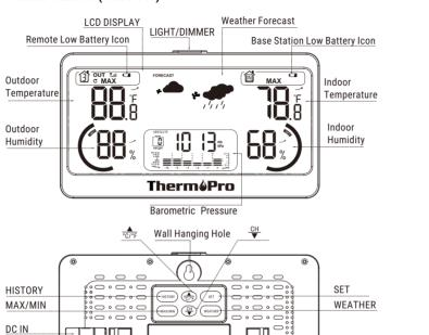
LIGHT/DIMMER: When the product is powered through the adapter, press the button to select among 4 brightness levels for the background light. (When the product is on battery-power, the background light will turn off after 15 seconds, and you can't select the brightness levels for the backlight).
