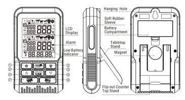
• LCD (Liquid Crystal Display) – Displays all icons, temperature and TIMER
